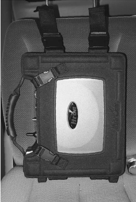
3. Tighten the straps until the RF unit is snug against the seat back.
